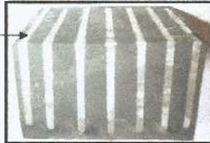
Tested Sample (Inner layer of Bearing Pad)
