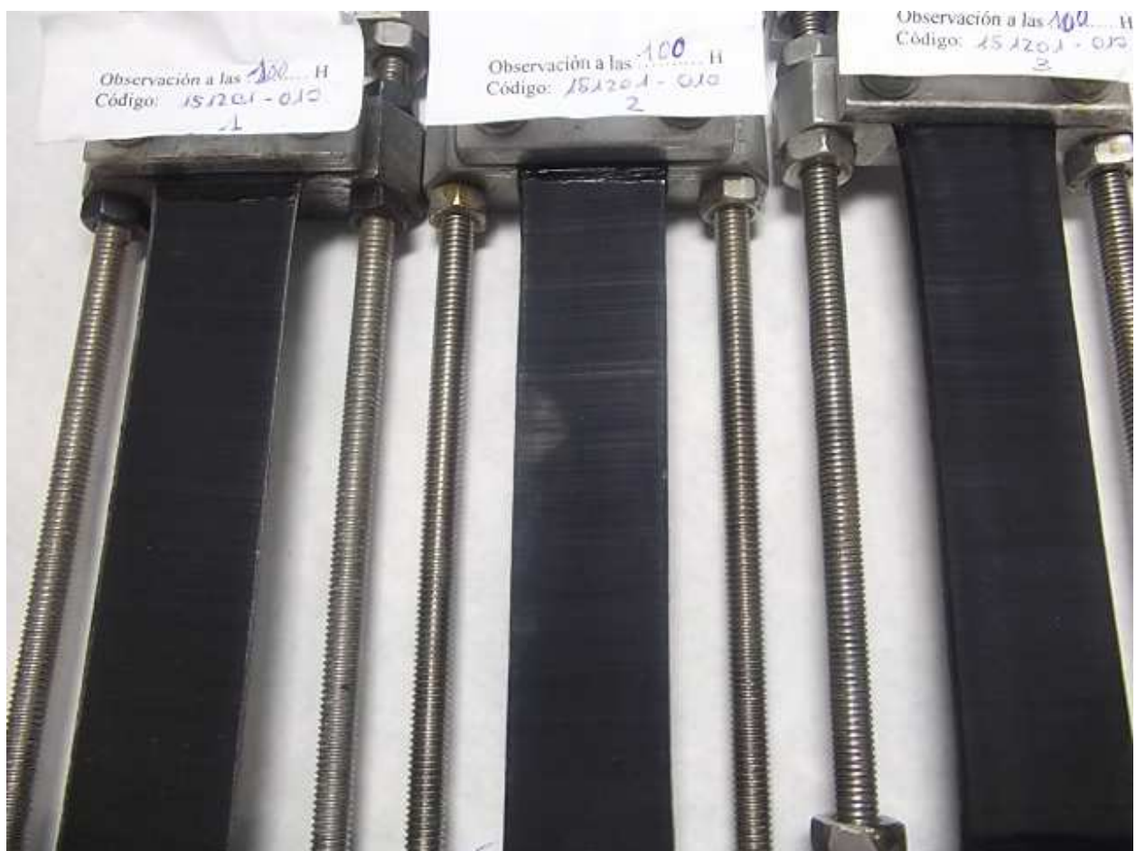
Test specimens after 100 of exposition to ozone
