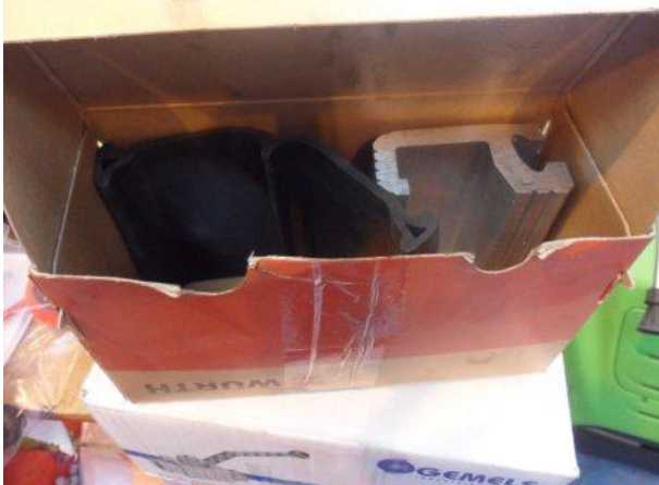
15. Samples of aluminium profile and elastomeric CR rubber profile SBJ-5 inside cardboard box
